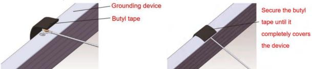
2. Schematic diagram of fixing the grounding clamp
