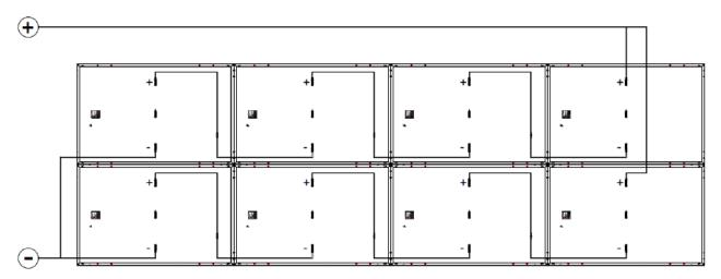
Allow modules in series to increase voltage or in parallel to increase current. In series, the positive electrode of the assembly is connected to the next negative electrode. In parallel, the positive electrode of a module is connected to the positive electrode of the next module.
