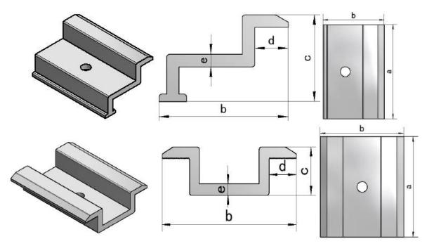
For customers with high load requirements, it is recommended to use a hook-shaped toothed press block that matches the module frame, and the thickness of the press block is at least 4mm. The specific size of the press block is shown below:
