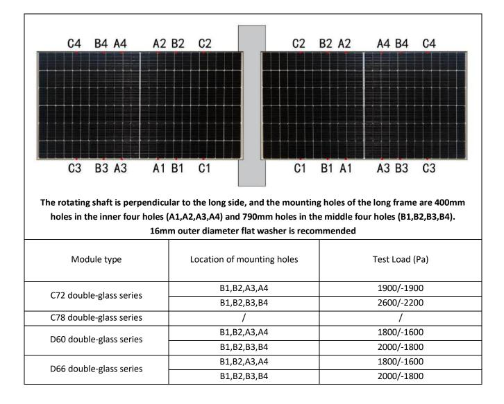
\* The above load values are based on the static load requirements in the IEC61215 standard (Suntech or third party certification body test).
