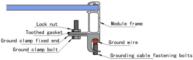
As shown in the diagram above, connect the copper conductor to the grounding hole on the module frame using the grounding components (M5 stainless steel cover bolt, M5 stainless steel flat washer, M5 stainless steel cup washer, and M5 stainless steel serrated nut).
