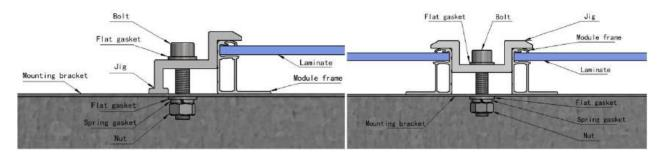
For structures where the mounting rail is parallel to the frame, overlap the assembly frame mounting surface and the rail by at least 20mm.
