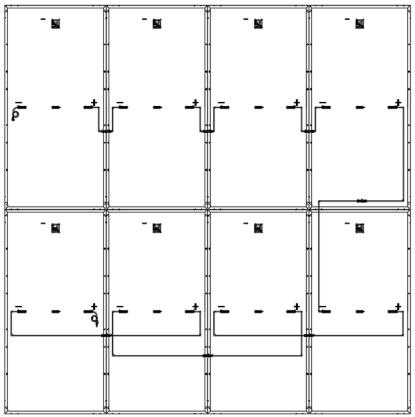
Modules in adjacent rows are flipped 180° to install: Series connection
