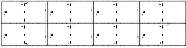
Modules in adjacent columns are flipped 180° to install: Series connection
