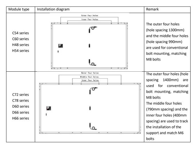
Suntech PV module bolt installation method is shown in the following figure:
