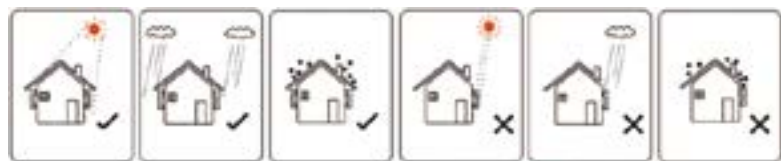
Figure 4-1 Recommended installation location
